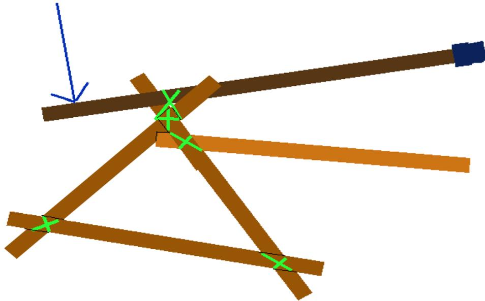
Shear lashing should be used for the top of the A frame.
