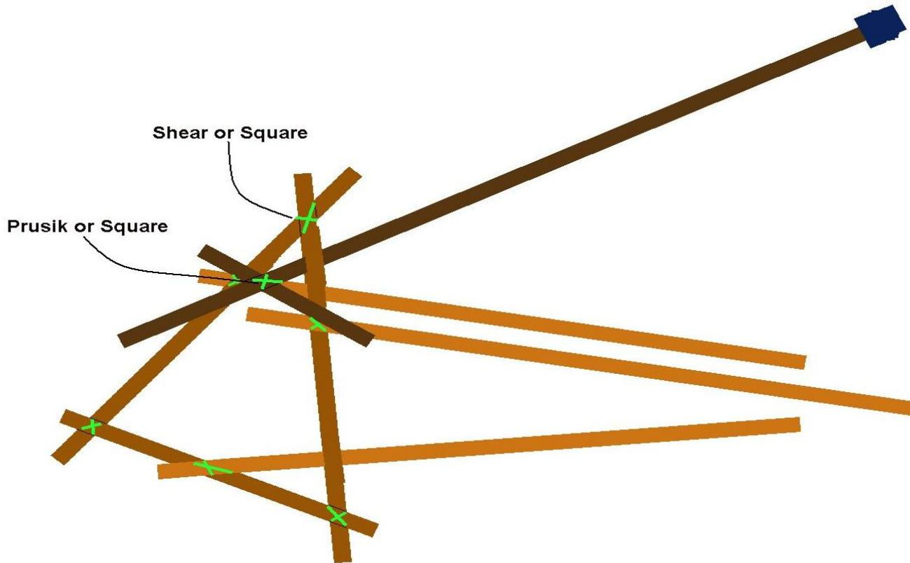
Shear lashing should be used for the top of the A frame. For other lashings use Prusik.
